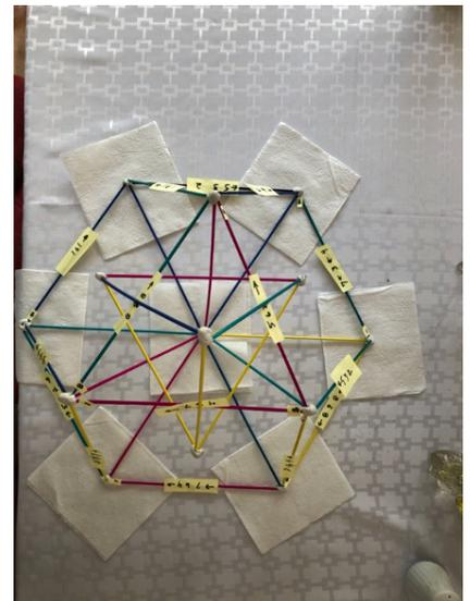
**Figure 43:** Two Orthogonal Vector Equilibrium Structures
